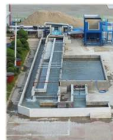
b) Development of unsteady flow hydraulic experimental equipment
